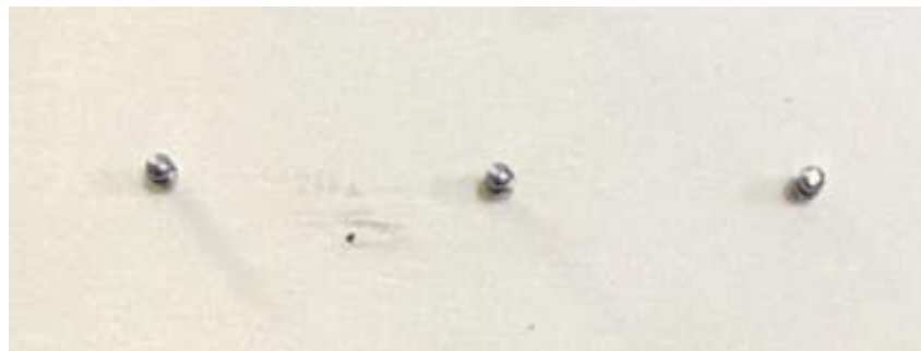
Fig 7: Modern Orthodontic implant places in 40 PCF artificial bone block at 90°
