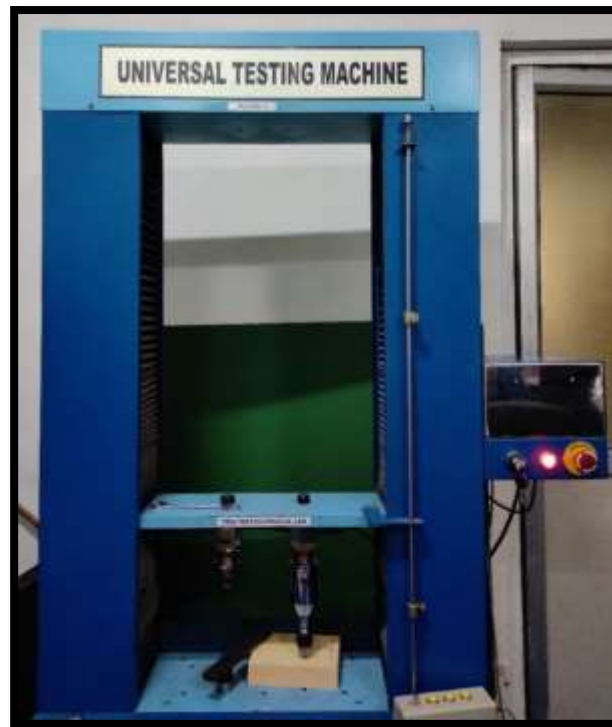
Fig 6: Universal testing machine
