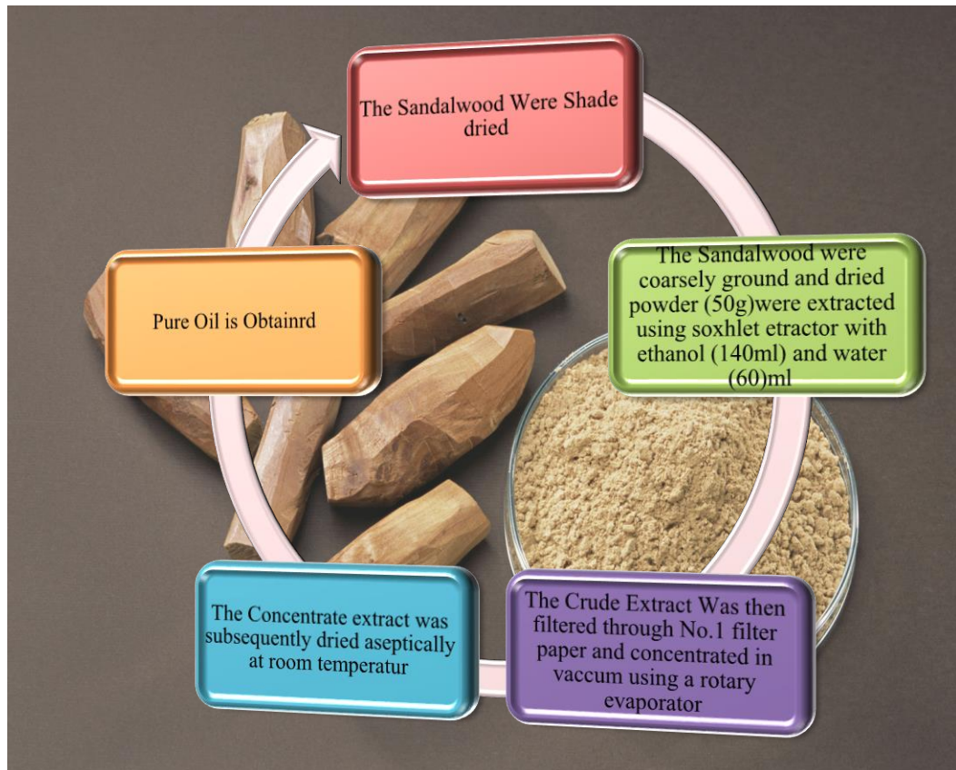
Fig. No. 1: Extraction Of Natural Oil By Soxhletion
