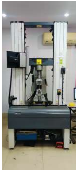
Figure 4: Universal Instron testing machine
