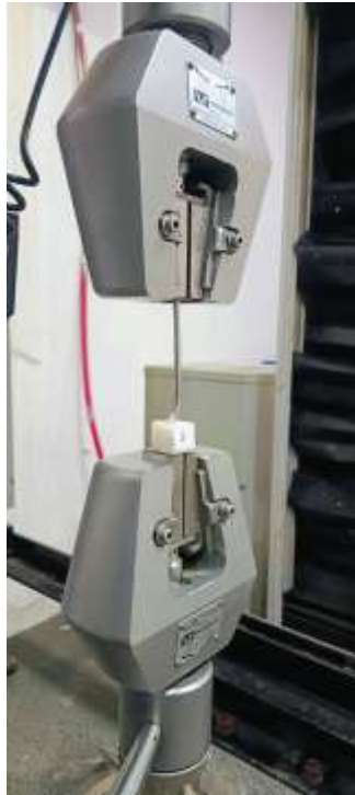
Figure 5: Measuring Of Shear Bond Strength.
