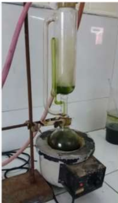
Figure 3.2: Soxhlet Apparatus Used for Extraction of Epipremnum aureum
