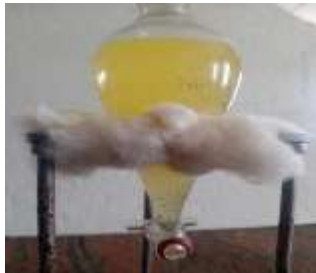
Figure8 Separating glycerol from ethanol-biodiesel
