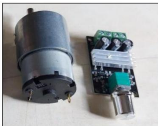
Fig. 8 High Torque Motor and PWM Controller
