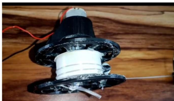
Fig. 17 Puller Mechanism Developed
