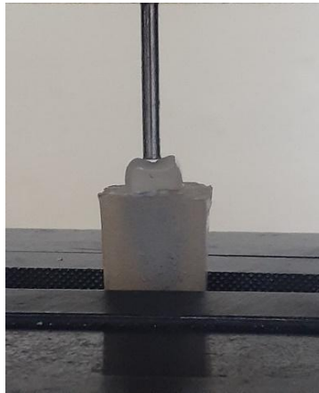
Sample in Universal testing Machine for fracture testing
