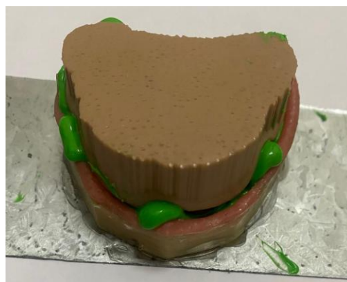
Figure 7B. front view of the printed key after load application
