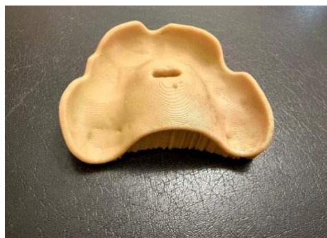
Figure 4 B. printed Key intaglio surface.
