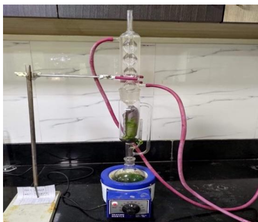
Fig:3 Crude plant extract by Soxhlet extraction Method.
