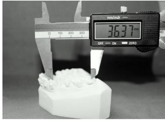
Figure 3: Measurements of space closure with a calibrated Digital Vernier Caliper
