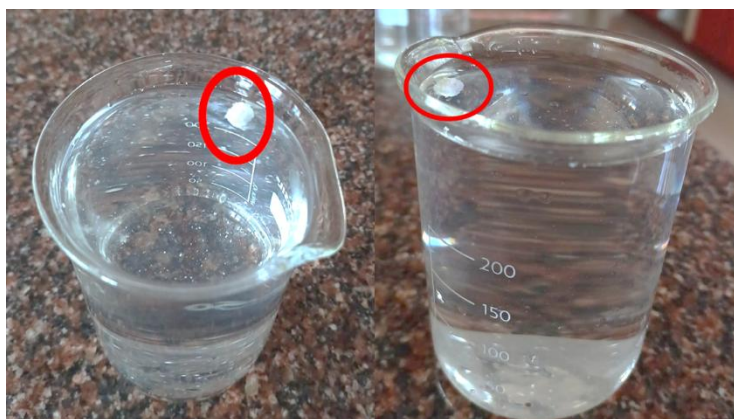
Figure 4. Determination of floating lag time and total floating time of the formulations prepared.
