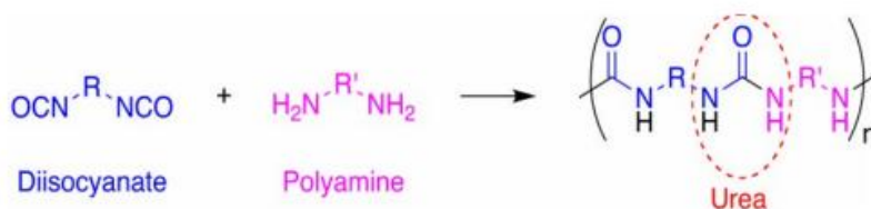
Figure 4: Overall response for the formation of a polyurea chain
