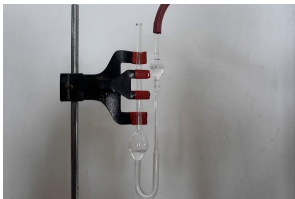
Figure 3- Determination of Density by Ostwald Viscometer
